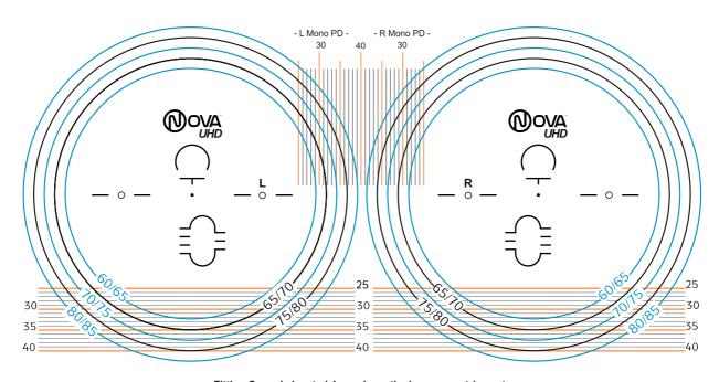
Fitting Cross is located 4mm above the lens geometric center
